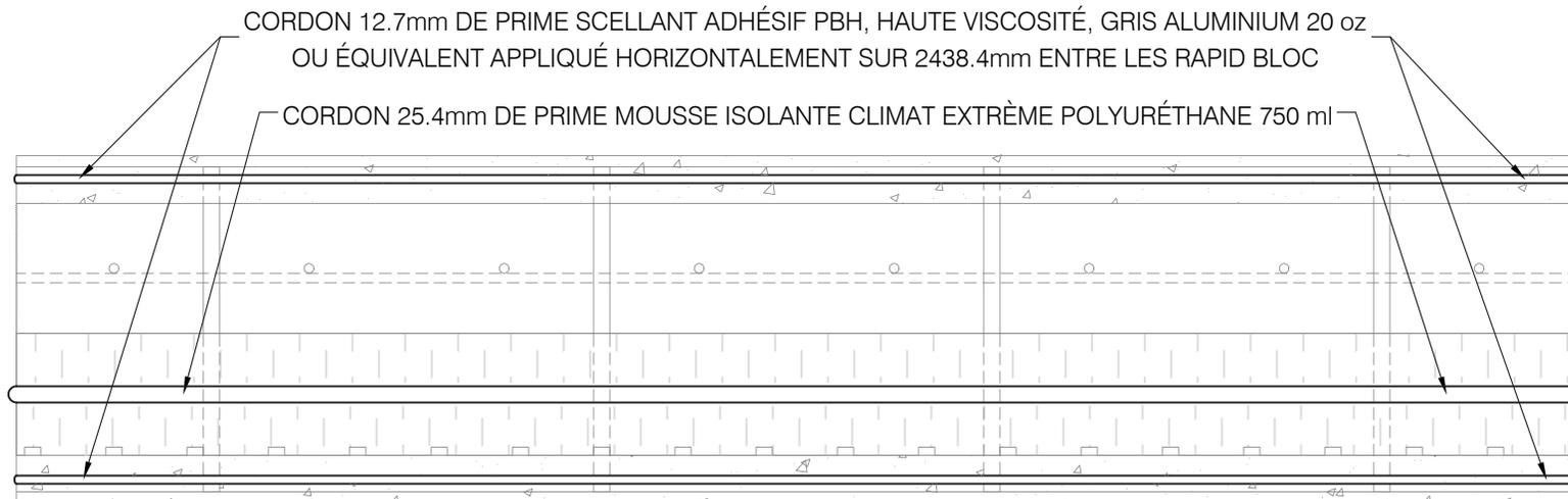
CORDON 12.7mm DE PRIME SCELLANT ADHÉSIF PBH, HAUTE VISCOSITÉ, GRIS ALUMINIUM 20 oz OU ÉQUIVALENT APPLIQUÉ HORIZONTALEMENT SUR 2438.4mm ENTRE LES RAPID BLOC
